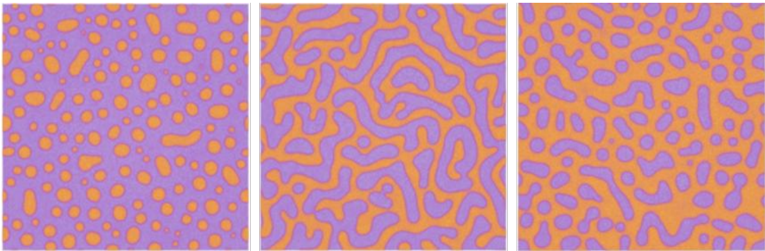
Figure 5.1: Simulation results displaying the three morphologies of interest: discrete (left), 2D bicontinuous (middle), and bicontinuous or porous (right). Images shown are at \tau = 2500 for nz = 20 with \phi_{NW} = 0.2, 0.275, 0.325 (listed left to right).
